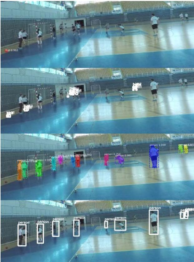
Figure 15. Indoor detection using (starting from the top) custom Mask R-CNN and YOLO following pretrained ones
