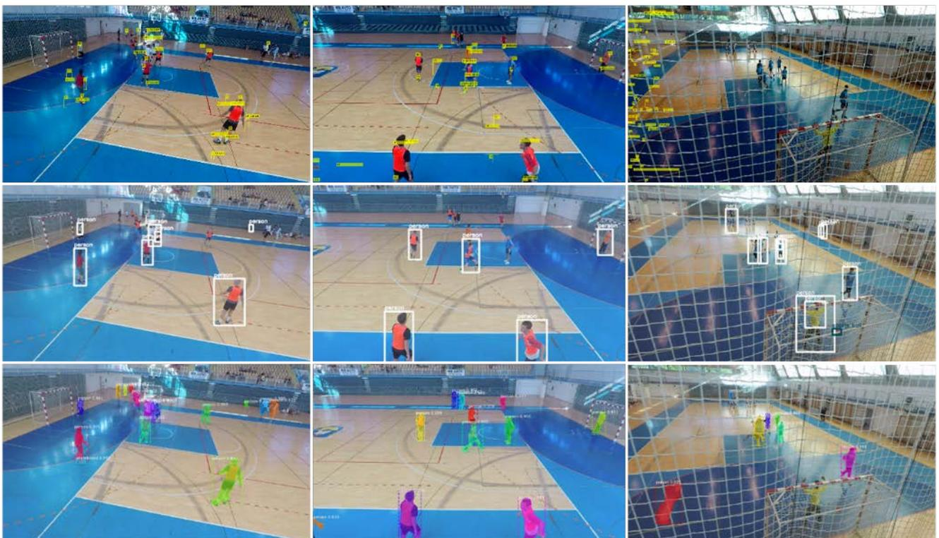
Figure 10. Indoor sport detection results of MOG (upper row), YOLO (middle row) and Mask R-CNN (lower row)
