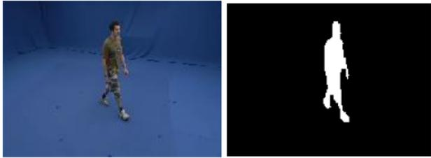
Figure 3. A video frame depicting a person walking (left) and the corresponding silhouette mask (right)
