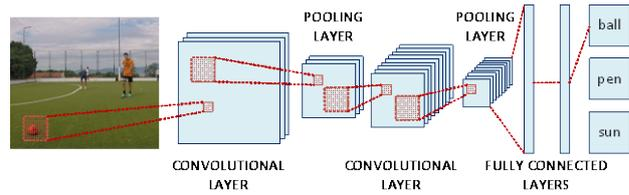
Figure 7. Typical convolutional neural networks
